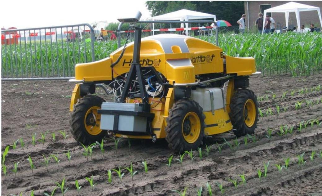
**Figure 4** "Hortibot" is an autonomous plant nursing robot that can control weed efficiently (Source: [www.hortibot.dk](http://www.hortibot.dk)).
